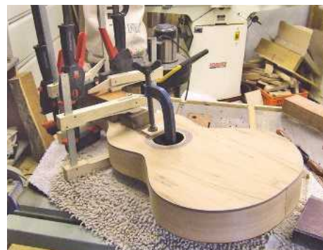
▲ Pic.23 Glue the fingerboard in place using cauls to spread pressure and prevent damage to the delicate structure
